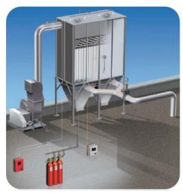
A pre-engineered fire suppression system is a packaged system which provides all the necessary parts and components to suppress fires in vessels before a deflagration event.  $CO_2$  is used as the extinguishant for organic, carbonaceous, plastic and chemical dust hazards, and Argon is used for metal dust hazards.
